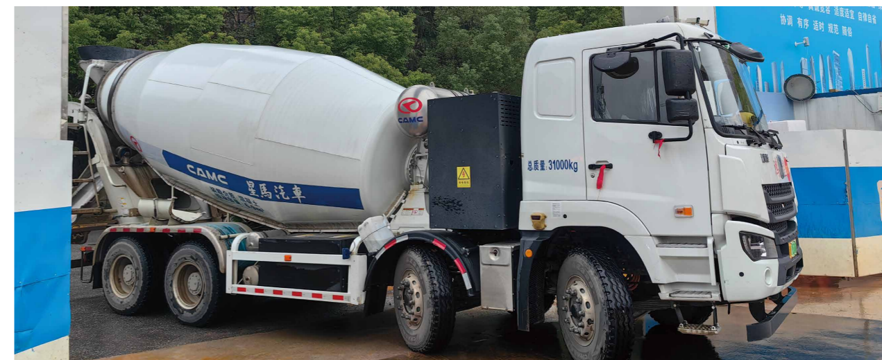
New energy vehicle for concrete transportation
